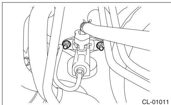
8) Remove the bolts and nuts which secure the brake pedal and clutch pedal, and remove the pedal assembly.
