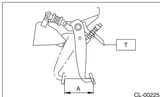
2) If the full stroke is not within the specified value, loosen the clutch switch lock nut to adjust.
